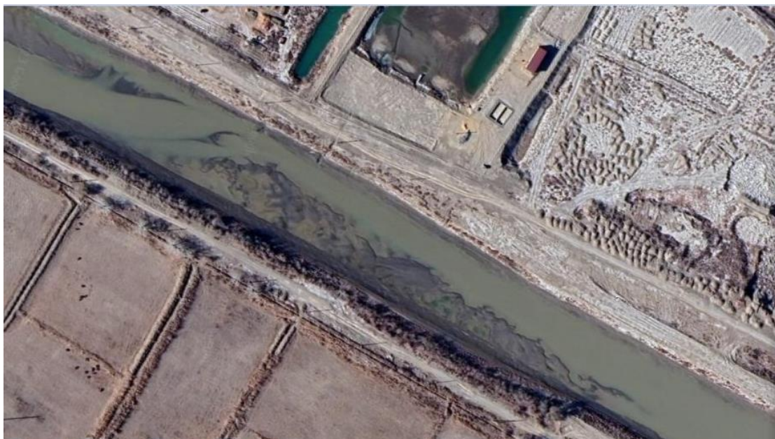
Fig. 3. Siltation and erosion in the Anasay main canal in the Republic of Karakalpakstan (2024)
